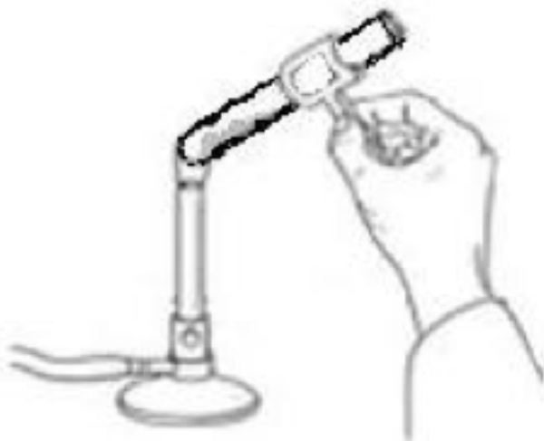
Figure 1: How to evaporate water from a hydrate.
