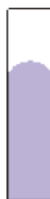
Figure 7.16b: Meniscus Mercury atoms do not interact well with glass, so the adhesive forces are very weak. Consequently, mercury forms a convex meniscus to maximize Hg-Hg interactions and minimize interactions with the walls of the container.
