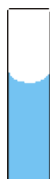
Figure 7.16a: Meniscus Glass contains many Si–O bonds, and water can hydrogen bond to the oxygens on the surface of the wall. The strong adhesive forces between water and glass tend to draw the liquid up the walls of the glass and produce the concave shape of the meniscus.
