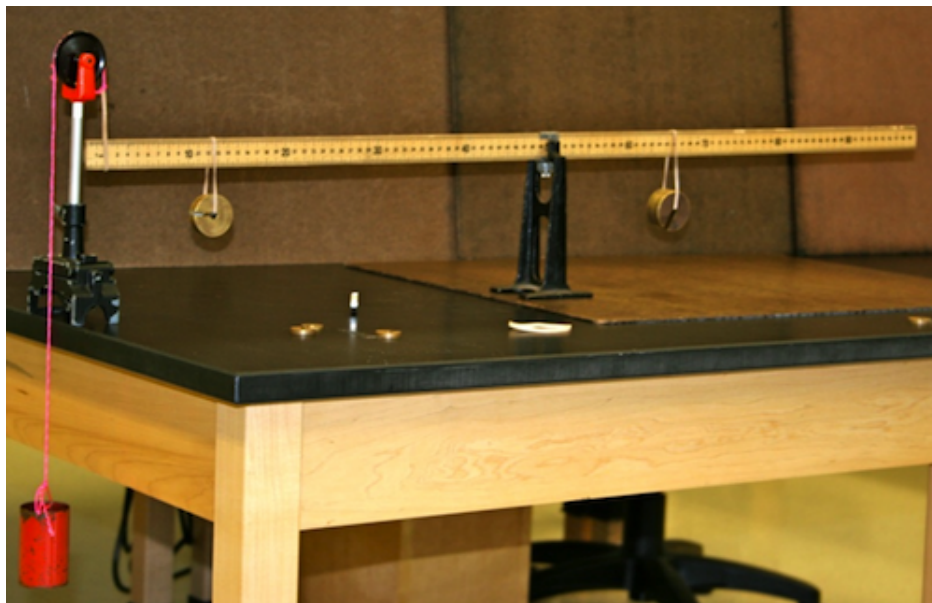
Figure 8: Photo of set-up for determining an unknown mass
