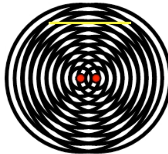
Figure 25.25: An interference pattern set up in a room by two speakers broadcasting identical single-frequency waves. For Exercise 4.
