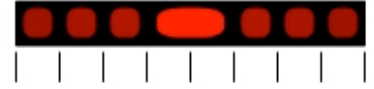
Figure 25.42: The pattern at the center of a screen, produced by a red laser beam shining on a single slit, a double slit, or a diffraction grating. The distance between neighboring tick marks, shown on the screen below the pattern, is 8.00 mm. For Exercise 49.
