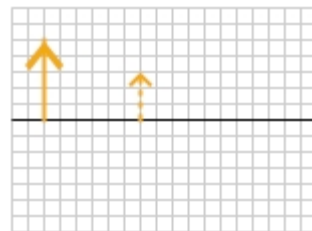
Figure 24.65: The larger arrow represents an object, while the smaller arrow represents the virtual image of that object, created by a lens. For Exercise 47.
