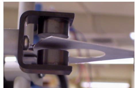
Figure 20.24: A photograph of the two magnets (dark cylinders) used to damp out the oscillations of the aluminum plate that is part of an apparatus used in a Coulomb's law experiment. Photo credit: A. Duffy.
