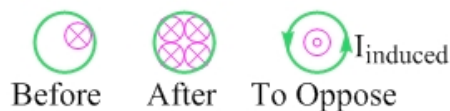
Figure 20.26: The pictorial method applied to the region that is entering the magnetic field.
