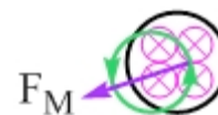
Figure 20.27: The magnetic force acting on the eddy current in the region moving into the field produces a torque that acts to slow down the wheel.
