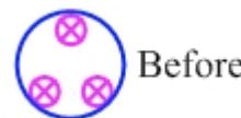
Figure 20.14: When the loop is in the Before position, the field from the long straight wire passes through the loop into the page.
