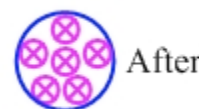
Figure 20.15: When the loop moves to the After position, coming closer to the wire where the field from the wire is stronger, we draw more field lines passing through the loop.
