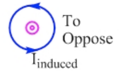
Figure 20.16: To oppose the change in flux as the loop moves from Before to After, the loop creates a magnetic field out of the page with a counterclockwise induced current.
