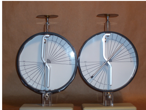
Figure 16.2: An uncharged electroscope, on the left, and a charged electroscope, on the right. Photo courtesy A. Duffy.
