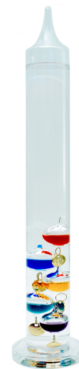
Figure 13.9: A photograph of a Galileo thermometer, for Exercise 37. Photo credit: Johanna Goodyear / iStockPhoto.
