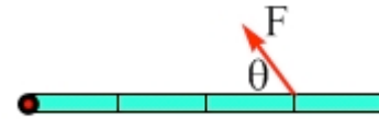
Figure 10.44: A side view of a rod that is hinged at its left end, and which is held in a horizontal position by an applied force F . For Exercise 50.
