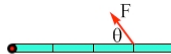
Figure 10.33: A side view of a rod that is hinged at its left end, and which is held in a horizontal position by an applied force F .
