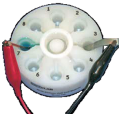
Figure 3: MicroLab Multi-EChem Half Cell module
