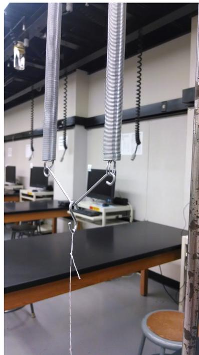
**Figure 7: System of springs in parallel**
