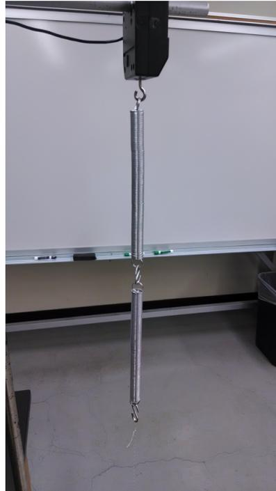
**Figure 6: System of springs in series**
