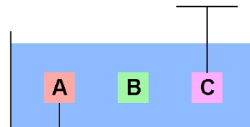
Figure 9.34: Three cubes of identical volume but different density at equilibrium in a container of fluid. For Exercise 40.
